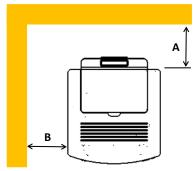
If the floor is made of combustible material, it is recommended to use protection made of non-combustible material (steel, glass...) that also protects the front from falling combusted material during cleaning operations.
