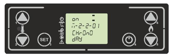
STOP2 Day. These slots can be defined according to the timings set out, where the OFF setting tells the clock to ignore the command. To modify, use P1 (to go up) and P2 (to go down). Confirm with P3. To go to next chrono set press P5 or P6.
