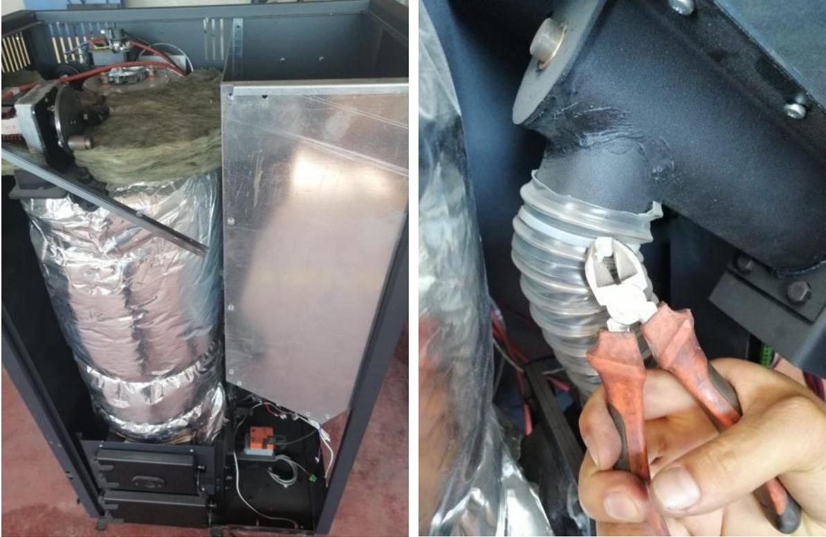
Remove real panel completely out of the boiler, then take the fuel tank outside the boiler. Use the A4 sized pattern supplied in fuel tank package to mark the correct place of the pellet sensor. See following picture.
