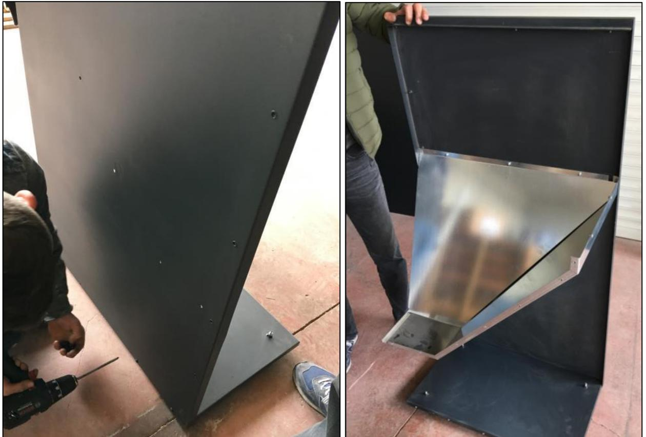
2.3. Fit right panel (4) and then rear panel (7) in order as seen in the following pictures. Fit front panel (8) (pellet inspecton glass is already installed on front panel)
