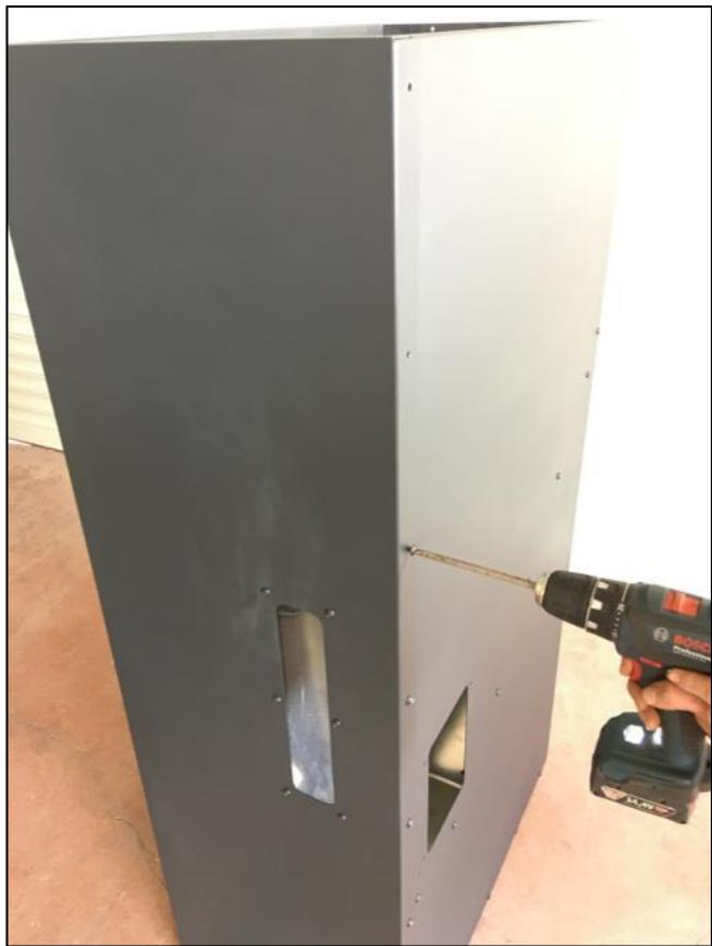
2.4. Fit feeding screw pipe support sheet (9) into the fuel tank, and fix it to the right panel with 4,2 x 13 self drilling SMS screw as seen in the following picture. Then fit service cover (10) onto the right panel with M5 x15 setscrews.
