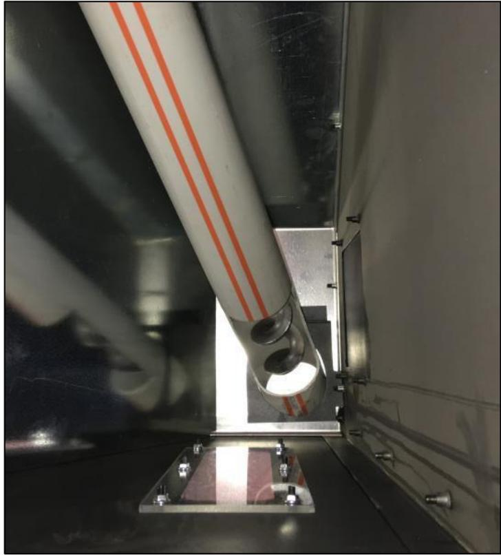
2.12. Fit pipe adaptor fixing sheet (23) onto feeding pipe adaptor (16) as seen on the following picture. Then, fix item 23 onto top panel of the tank (12) to keep the position of item 15 fixed for optimum pellet feed.
