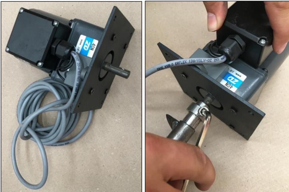
2.10. Pass feeding screw group through feeding pipe adaptor. Loose parts of Pg-11 cable gland, and, pass and secure the power cable of gear motor as seen on following pictures. Fix gearbox assembly plate to feeding pipe adaptor (16) by 4 sets of M5x15 pan head setscrews and M5 nuts.
